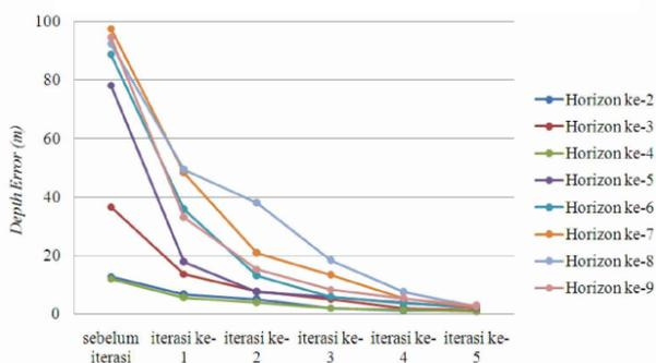
**Fig. 9.** Graph of the relationship between the number of tomographic iterations and the depth error of well 1 and after Tomography (1<sup>st</sup>-5<sup>th</sup> iteration)
