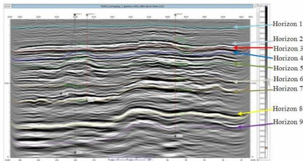
**Fig. 8.** The 2222 inline PSDM section results from running PSDM using the final interval velocity model (fifth iteration)
