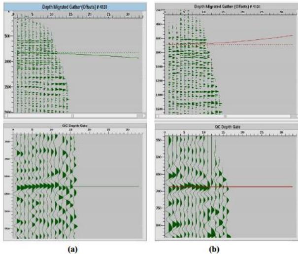
**Fig. 6** (a) positive *residual move-out* (event is bent down), which indicates that the velocity is too high, (b) negative *residual move-out* (event is bent up), which indicates that the velocity is too low.
